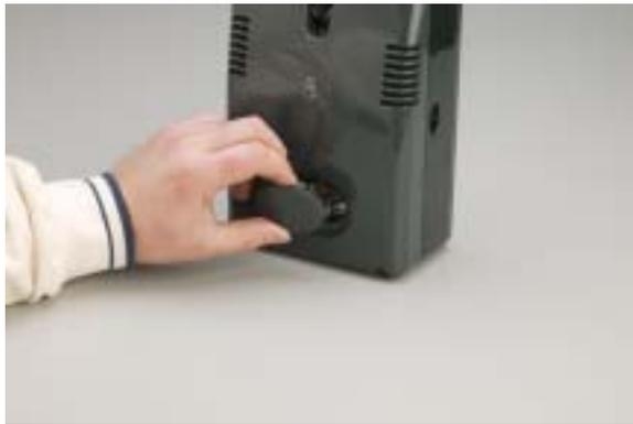
Figure 11: Removal of Air Intake Filter Cover
