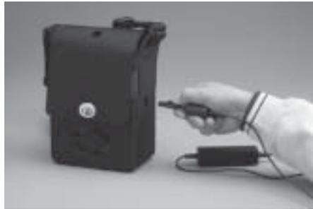
Figure 5: Internal Battery Charging
