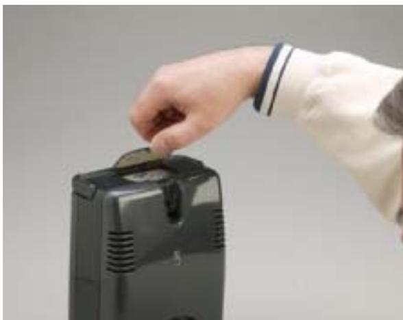
Figure 13: Lifting Dust Cover on Keypad Display
